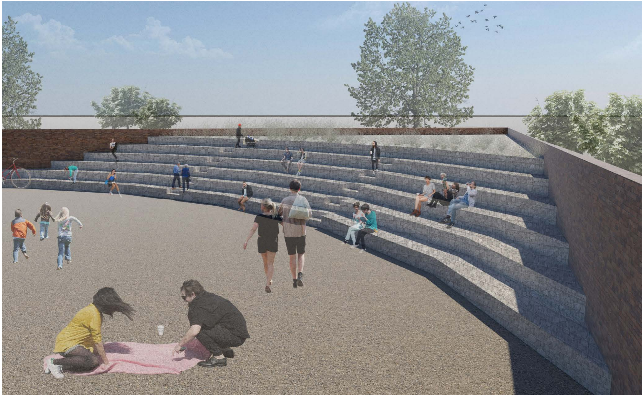
stacked gabion seating
